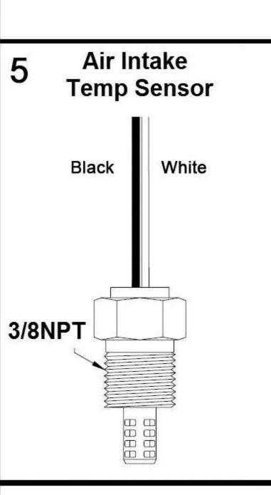
3/8 NPT weld-in bungs of the appropriate material are required to install the sensors onto the piping.
